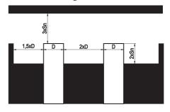
correction factors indicate the change relating to the sensing range if materials other than steel (1.0037) are used. The change in the sensing range depends on the type, characteristics (internal structure), size and the geometry relating to the material that is to be detected. In order to assess the approximate sensing range on the materials which differ from steel, the value for steel has to be multiplied by the appropriate correction factor.
