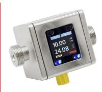
If an electrically conductive liquid moves across a magnetic field, a voltage is generated vertically to this magnetic field which is dependent on the flow velocity. This voltage is measured by electrodes located in the wall of the measuring tube. Micro-controllers evaluate this voltage, calculate the flow rate and show it on the display. An analog signal and a transistor switching output are available for further processing.
